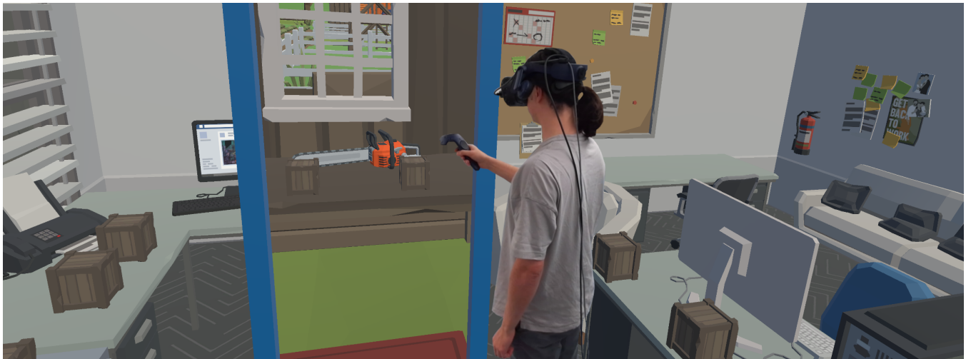
Figure 1: Some applications require switching between multiple environments. Here the user is using a Portal transition and is about to walk through the portal leading to the new environment (in the evaluation, a wireless headset was used).
